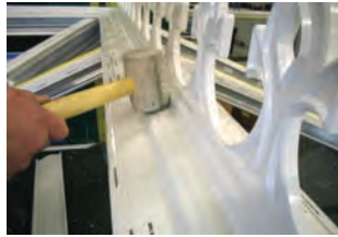
Starting at one end knock the top cap in to position using a rubber mallet.
